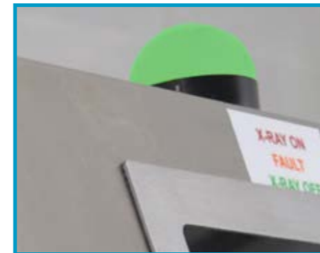
360° View Status light clearly displaying when x-rays are being generated
