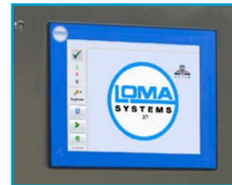
User interface provides access to key status information and multi-level user security prevents inappropriate use
