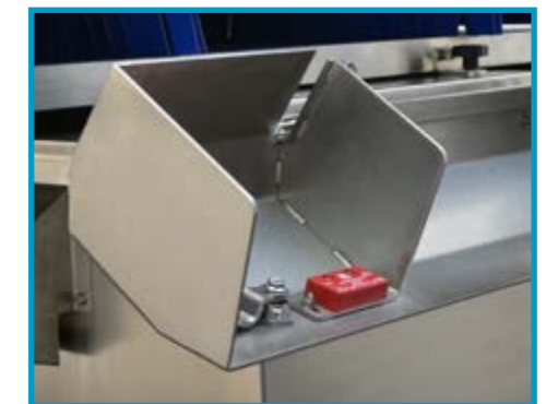
Lockable covers with safety interlocks to prevent X-rays being generated with the covers open
