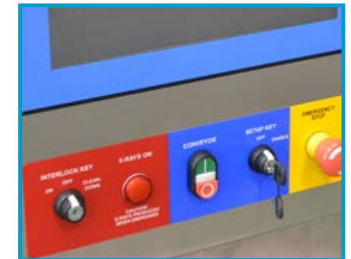
Critical controls are placed within operators reach
